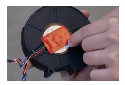
4. Carefully reinstall the fan into the shroud and press firmly to set the adhesive.
